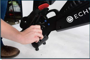
Step 13. Tighten screws with hex key. Repeat with left foot carriage.
