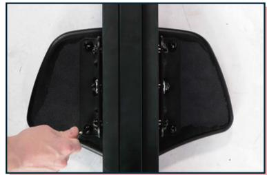
Step 6. Place all four screws (No.7) into screw holes and tighten with hex key.
