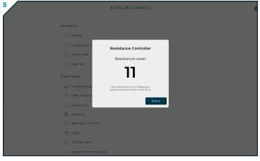
Test the connection by changing resistance via the Bluetooth Resistance Controller.
