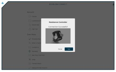
The Bluetooth Resistance Controller will flash solid blue lights once it is connected, and the app will say "Connection Successful!" (Lights do not flash during normal operation.)
