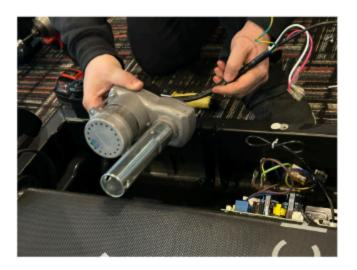
Step 8. Install the new incline motor, secure it with bolts, and reconnect all wires.
