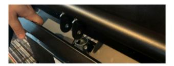
Step 5. After relocating the motor, you will uncover the incline motor. Initiate the process by extracting the bolt. While removing the bolt, remember to lift the motor and simultaneously push the bolt out.
