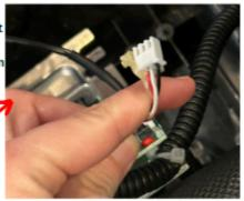
Step 7.Once the wires are detached, you can extract the incline motor. It might be easier if another person lifts the back of the treadmill.
