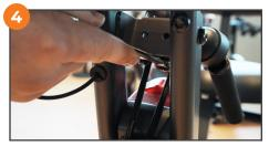
Use 10mm wrench to remove the nuts by working in conjunction with step 3.
