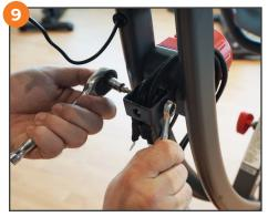
Use a 4mm hex head and 10mm wrench to loosen and remove hardware around pulley wheel.
