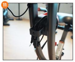
Place the new bands before reassembling the pulley onto the bike.
