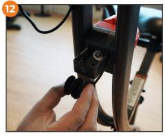
Re-insert wheels and hardware. DO NOT overtighten the bolt and nut on the pulley wheels.
