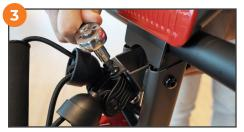
Use a 4mm hex head with a 1/4" socket wrench to loosen the bolts. Do this in conjunction with step 4.
