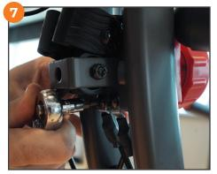
Use 4mm hex head with the 1/4" socket wrench to loosen screws.
