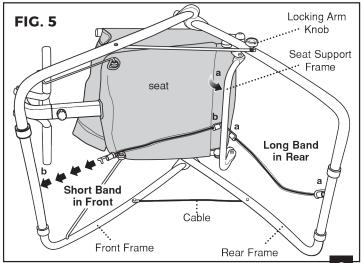
other end of Long Band to hole on Rear Frame (a). Make sure hooks are inserted completely (fig. 5c). NOTE: Chair will pivot easily at this point. Make sure you hold Frame firmly in place as you attach bands.
