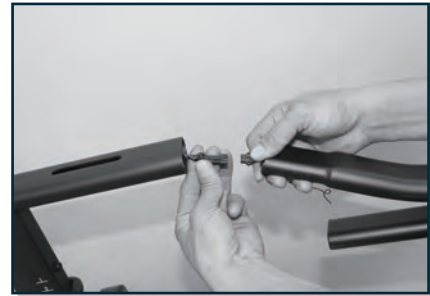
Connect the wire from the handlebar post to the wire at the bottom of the tablet mount.
