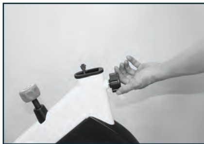
Unscrew handlebar post adjustment knob, but do not remove.
