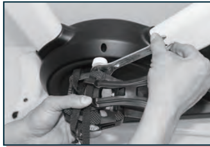
Use the double sided wrench to ensure pedal is firmly seated against crank arm.
