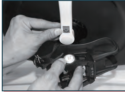
Match pedal and crank arm marked with 'R' label.
