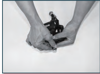
Remove nut from right pedal by turning counterclockwise .
