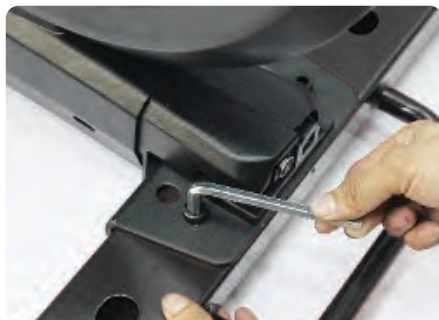
Tighten bolts with 8mm Allen Wrench.
