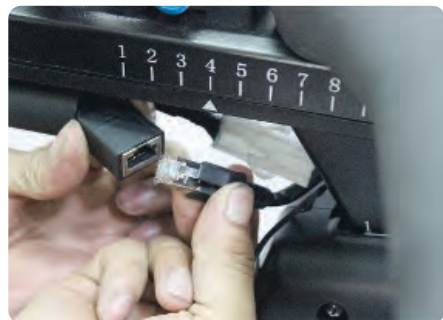
Connect the ethernet cable.
