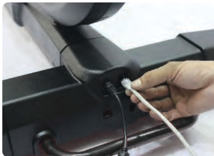
Insert the ethernet cable at the rear or front foot.
