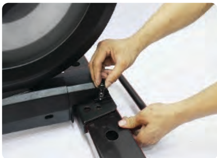
Line up the holes and finger tighten with (2) M10×25mm foot bolts.
