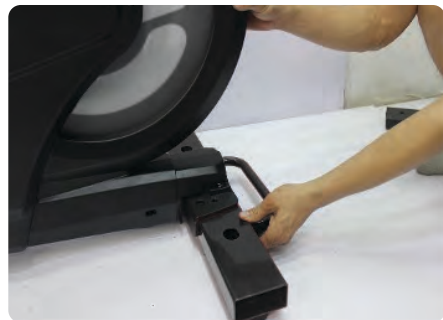
Lift the main body and assemble rear foot.
