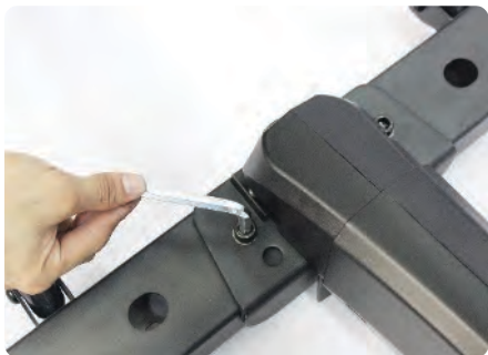
Tighten bolts with 8mm Allen Wrench.
