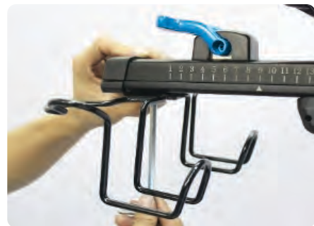
Tighten the bolts with the Phillips Head screwdriver end of the 6mm Allen Wrench.
