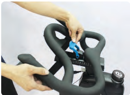
Push down the handlebar lever until secure.
