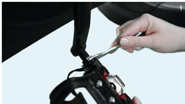
It is important to ensure pedals are installed properly and routinely tightened.
