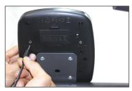
Connect heart rate wire to the control panel.
