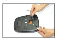
Remove screws from the back of the control panel.
