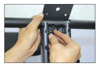
Place screws into holes and finger tighten.
