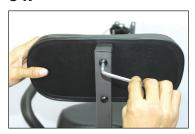
Tighten down screws with included large hex key/screwdriver tool.
