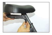
Insert screw through hole in backrest support.
