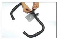
Remove screws from handle bar.
