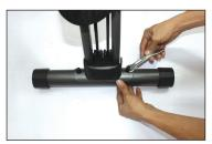
Tighten nut onto screw with included wrench. Repeat on other side.
