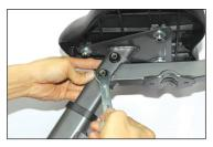
Place nut on screw and finger tighten. If difficult to tighten, nut may be upside down. Tighten fully with included wrench.
