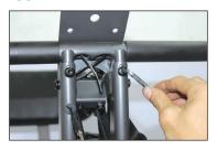
Tighten down screws with included small hex key tool.
