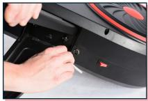
2. Tighten the screws with hex key.
