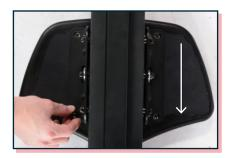
4. Place seat on ground and lay the rail onto seat so the screw holes on the bracket align with screw holes on seat.
