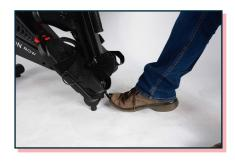
To lower the rail, press down the foot pedal at the joint and lower the rail gently to the ground.
