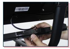
Place power cord in the notch of the middle perforated section of the cover and hold in place.
