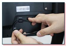
Plug in power cord to DC input and place excess cord in wire clip.
