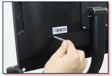
Replace the three screws to secure the cover back on the tablet.
