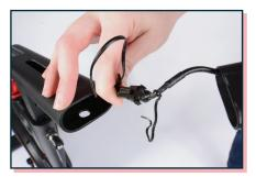
Untie the twist tie at top of handlebar post, ensuring not to allow the wire to fall inside of handlebar post. Connect the wire from the handlebar post to the wire at bottom of screen mount.
