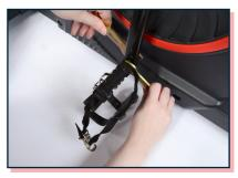
Hold pedal with double sided wrench and use single sided wrench to tighten nut clockwise.
