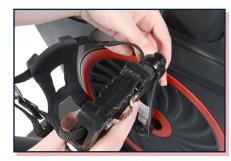
Finger tighten nut counterclockwise back onto pedal bolt.
