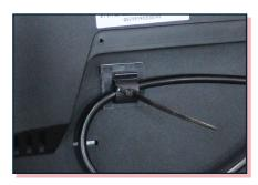
Pull zip-tie to tighten and secure cord in place.
