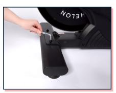
Tighten down foot bolts with included hex key.
