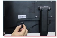
Place wire clip, as shown above, and press and hold wire clip down for ten seconds for proper adhesion.
