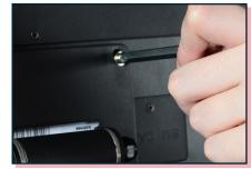
Flip mount around to face away from Connect bike. Hold tablet up to mount and hand screw all four screws into tablet. Use screwdriver end of hex key to tighten.
