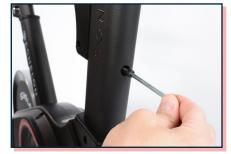
Insert handlebar post screw into hole on post. Use small hex key to tighten. Ensure holes in handlebar post and handlebar post frame align properly before inserting handlebar post bolt.
