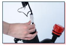
Connect the one wires from frame and handlebar post together, then feed excess wire down into frame.
