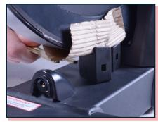
Use a pair of scissors or wire cutters to cut zip ties around wheel chocks. Using one of the wrenches, knock out the front then the back chock.
